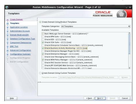
For BPM enabled domain (\_If BPM process flows deployment is required then we have to select the Oracle BPM Suite – 12.2.1)
