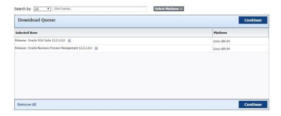
**NOTE (Doc ID 1904280.1)**: As part of the new Release of SOA 12c, you need to get WebLogic 12c through the Oracle Fusion Middleware Infrastructure installation, which contains all required components for SOA. The standard WebLogic 12.2.1.0.0 Installer i.e. fmw\_12.2.1.0.0\_wls.jar, does not have the required JRF templates.
